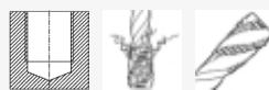
blind holes up to 2,5 x D Chip removal (like picture) Form C 40° spiral flute
