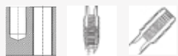
through holes & blind holes up to 2 x D Chip removal (like picture) Form C straight flutes
